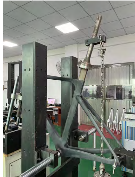
Figure 3.4: Seattube Fatigue Test.
