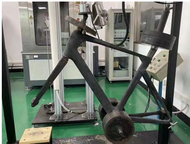
Figure 3.5: Frame Impact Test.
